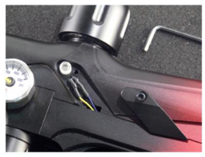
1. Remove the eye cover by unscrewing the 4-40x1/4 SHCS.
