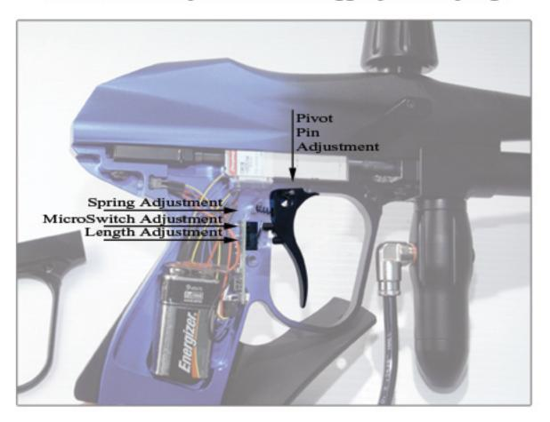
This drawing is for illustration. You may adjust any of the three set screws without removing the clamshell grip frame. However, to adjust the pivot pin, remove the clamshell.
