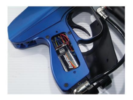
Orient the marker so that the barrel faces to the right. Remove the two grip panel screws on the right side of the marker.
