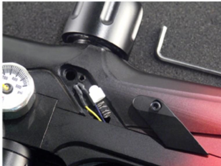
**2. Clean the ball detent with water and dry thoroughly. Clean the area around the ball detent if needed. Do not lose the small spring.**
