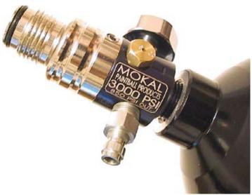
This picture shows the regulator separated from the tank. In this case **the tank should not be removed.** There is a vent hole located in the tank thread that will vent out the air in the tank if the regulator unscrews from the tank. Allow the air in the tank to completely escape before attempting to remove the tank. You should have your tank serviced by a qualified air smith to properly remove the tank and reinstall the regulator.
