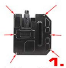
Using a phillips screwdriver, loosen the 6 screws and take off cover.
